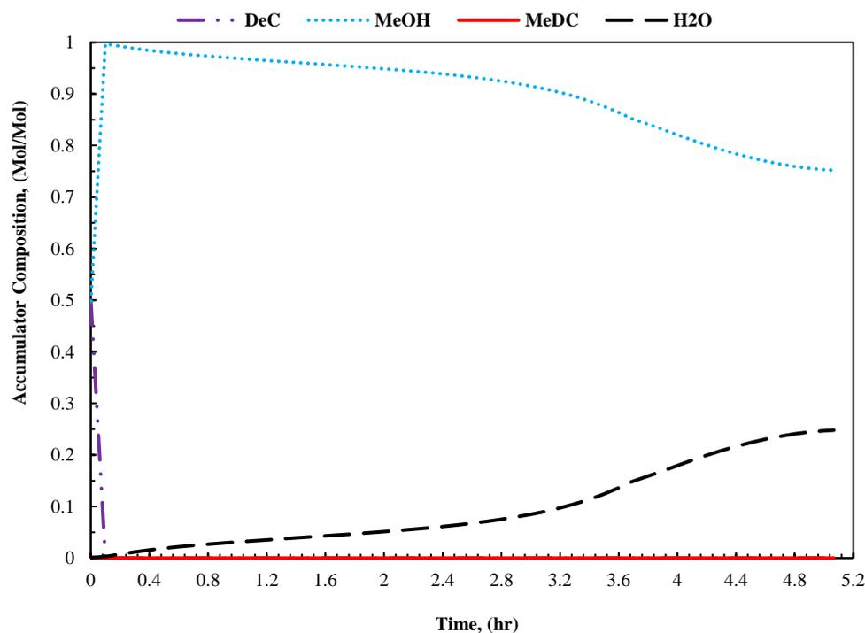
Figure 4: The accumulator composition profile for SBD, Two Intervals Control ( $x_{\text{MeDC}}^* = 0.945$ ).
