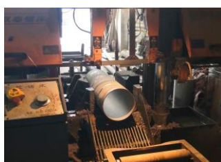
(a) Bench saw for cutting
