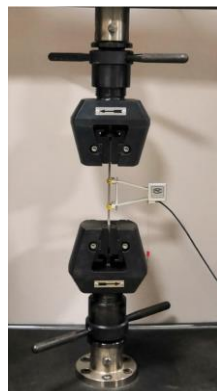
(a) Tensile coupon test-setup
