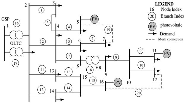
Fig. 1. 16-bus UKGDS meshed with candidate locations for PVs
