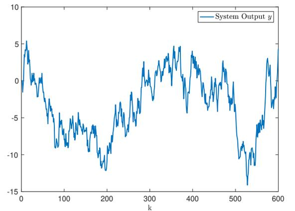
Fig. 12. The output of the twin-tank level process control system around the equilibrium which is  $23cm$ .
