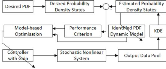
Fig. 4. Block diagram for the data-based output PDF control via indirect optimisation while the PDF dynamics have been represented by an identified model with probability density states.
