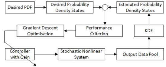
Fig. 3. Block diagram for the data-based PDF control via direct optimisation.
