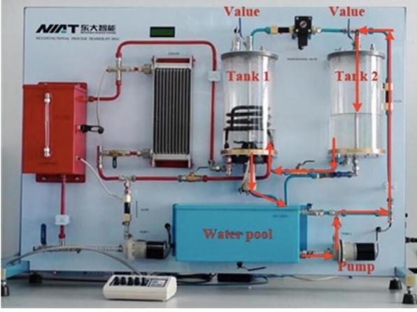
Fig. 9. The structure of the twin tank level process with interconnection.
