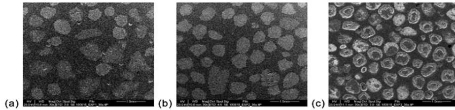
Figure 3: SEM images 30 $\times$  of granules at constant 10 % of binder; (a) Powder ratio of 3 (75 % Fine: 25 % Coarse), (b) Powder ratio of 1 (50 % Fine: 50 % Coarse), and (c) Powder ratio of 1/3 (25 % Fine: 75 % Coarse)
