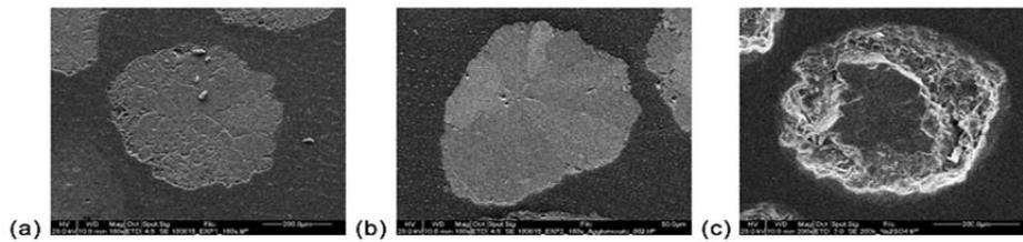
Figure 4: SEM images 200 $\times$  of granules at constant 10 % of binder; (a) Powder ratio of 3 (75 % Fine: 25 % Coarse), (b) Powder ratio of 1 (50 % Fine: 50 % Coarse), and (c) Powder ratio of 1/3 (25 % Fine: 75 % Coarse)
