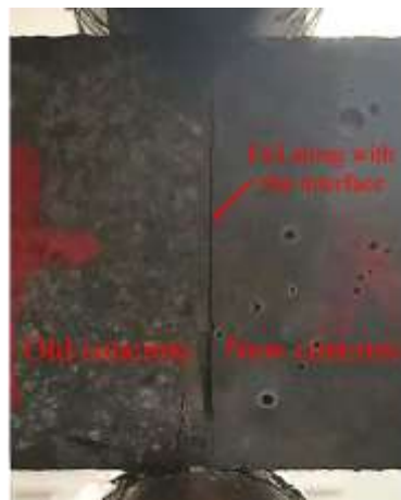
Figure 2. Representative failure form
