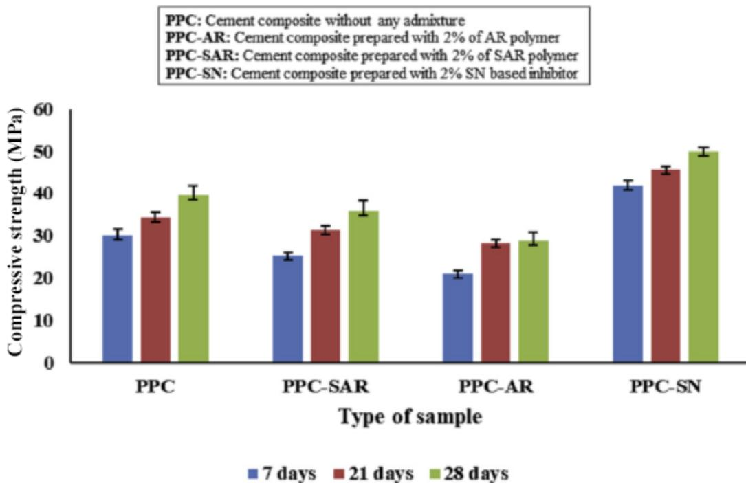
567 Fig. 8 Comparison of compressive strength of (SAR denotes styrene acrylate
