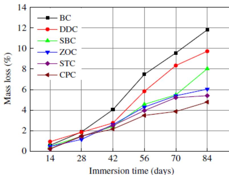
569 Fig. 9 Effect of various bactericides on mass loss of concrete immersed in sewage
