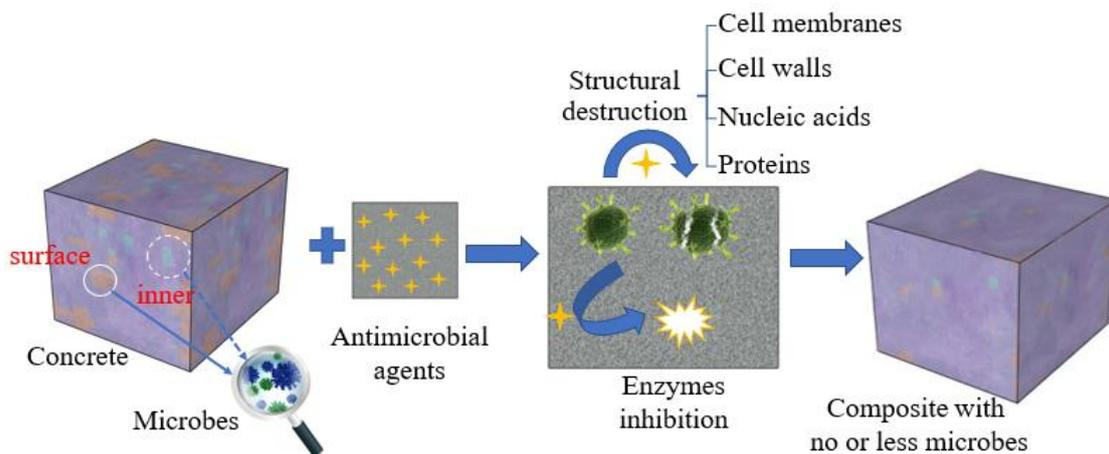
122 Fig. 1 Schematic diagram of antimicrobial concrete.
