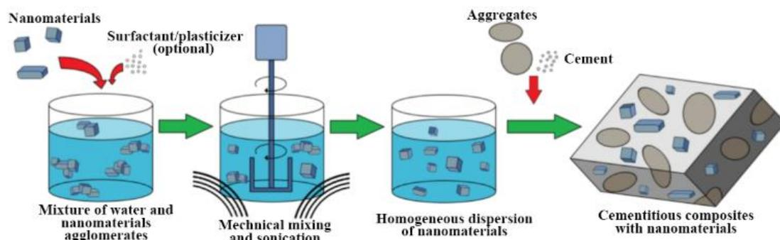
208 **Fig. 2** Schematic process of nanomaterials dispersing method commonly used in
