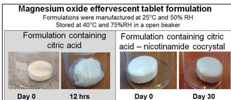
**Figure 2.** Comparative stability of magnesium oxide effervescent tablet containing free CA and CA-NIC co-crystal as part of effervescent mixtures
