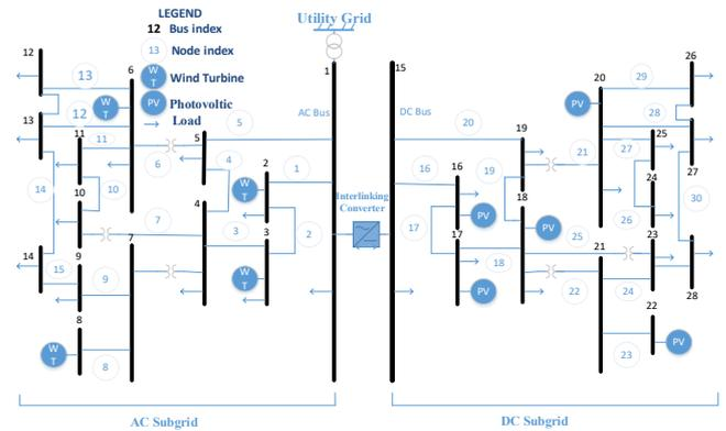
**Fig.5.** Single-line diagram of real Hybrid ac-dc microgrid
