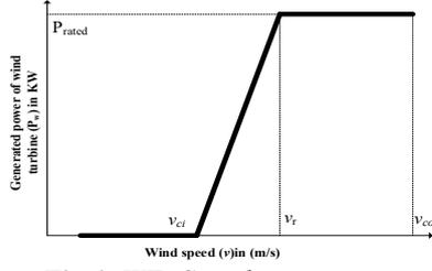
**Fig.1.** WT's Speed power curve.
