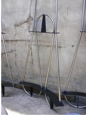
(a) The W serpentine shape tube heat exchanger.
