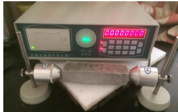
Fig.6 Longitudinal fundamental frequency testing device
