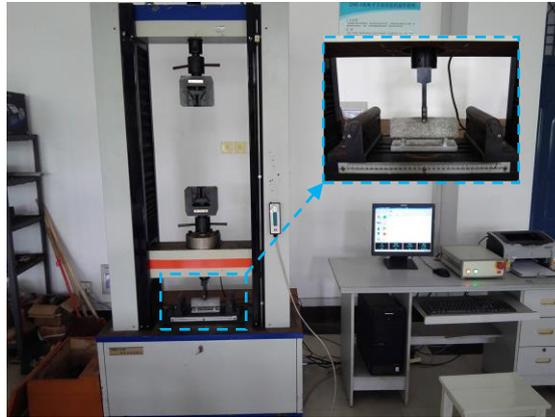
Fig.10 Flexural test
