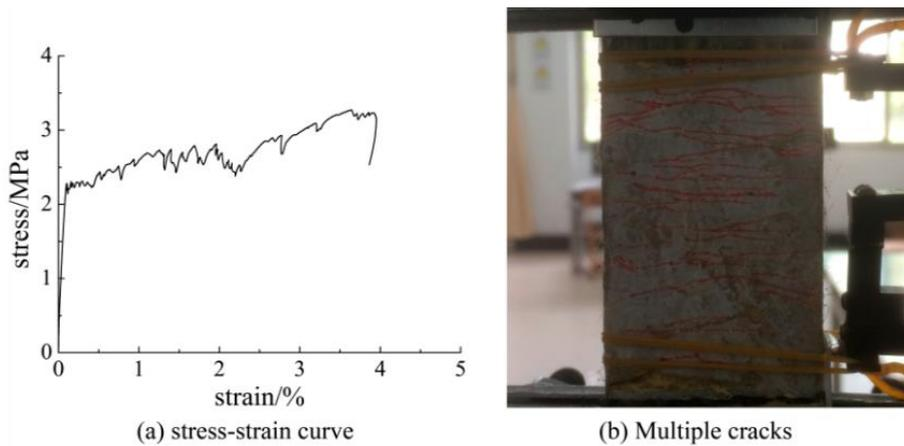
Fig.1 Typical characteristics of ECC
