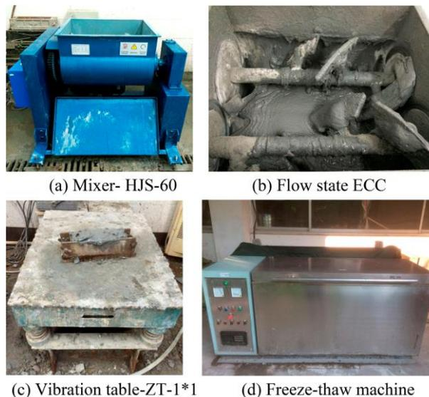
Fig.3 Testing Machines
