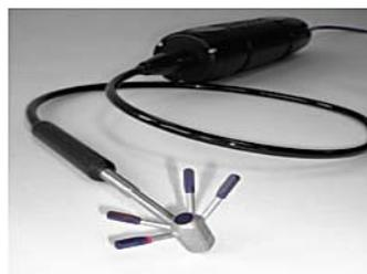
Figure 2. Side-Looking ADV probe
